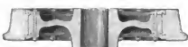
Figs. 4557-4558. No. 1 Krupp Wheel. Wrought Iron Coil Disc Center. Tire Secured by Wrought Iron Retaining Rings.
